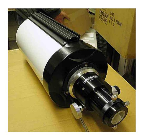
Pictures below areof the VRC 12 - a Video Ritchey Chretien Optical Tube mounted on a Losmandy Titan Equatorial Mount. The images were taken from the MallinCam Observatory in downtown Ottawa Canada.
