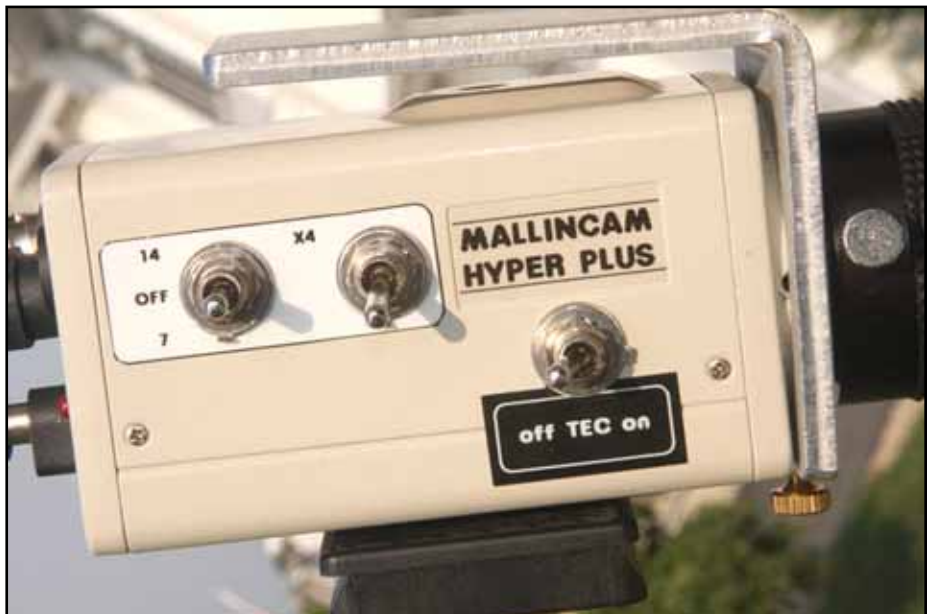
Top and Middle: Laptop and connections for imaging with the Mallincam Bottom: All hyper switches are turned off including the TEC cooler
